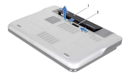
battery 2 1 battery release latch
